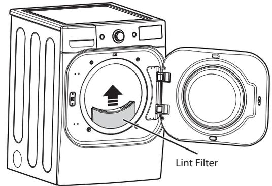
To clean, open the dryer door and pull the lint filter straight up. Then:
