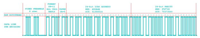
Figure 2. PPM-encoded ADS-B 56 bit sample frame.
