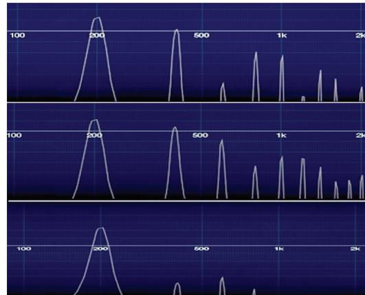
**Figure 5.** Output from a Bugera BC15 amplifier. Top: moderately overdriven preamp valve; middle: strongly overdriven preamp valve; bottom: weakly overdriven transistor power amp.
