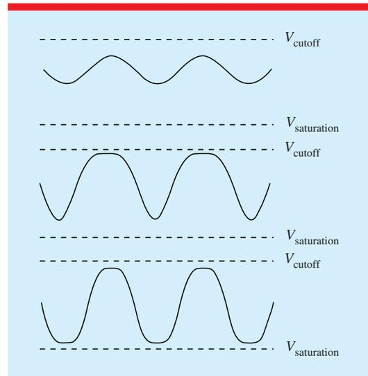
**Figure 8.** Expected output wave shapes when a sine wave of increasing amplitude is input to the cathode-grid circuit. Top: linear amplification before either plate voltage limit is reached; middle: an asymmetric wave as one plate voltage limit is approached; bottom: a symmetric wave as the second limit is approached.
