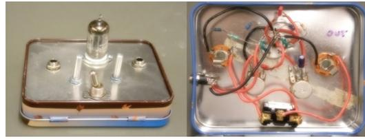
**Figure 10.** ValveLiTzer® overdrive pedal.
