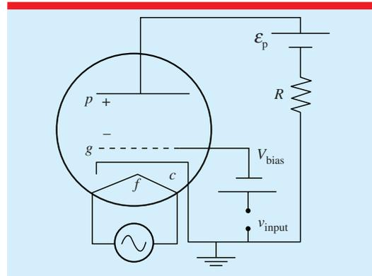
**Figure 7.** A triode valve functioning as a voltage amplifier.
