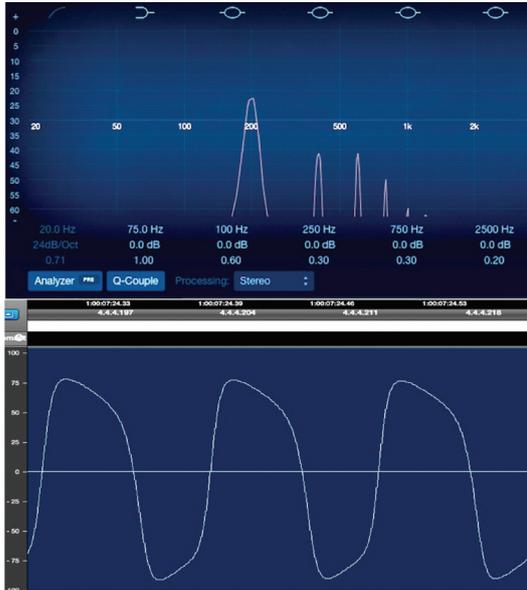
**Figure 3.** Amplifier output displayed by Logic. Top in frequency domain, bottom in time domain.
