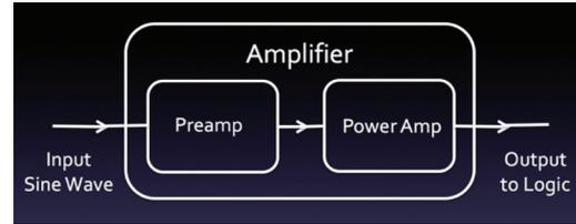
**Figure 4.** Amplifier overdrive test: input a sine wave, increase preamp or power amp gain, and view frequencies or wave shape using Logic.
