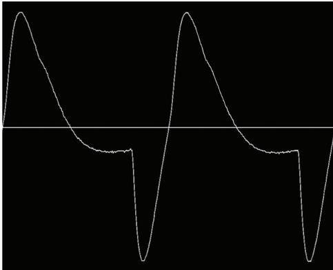
**Figure 9.** Output wave shape from a Bugera BC15 amplifier with its valve preamp overdriven.
