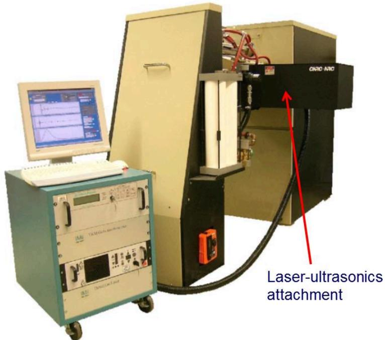
Figure 32: Laser-ultrasonics coupled to a Gleeble <sup>TM</sup> 3500 thermo-mechanical simulator
