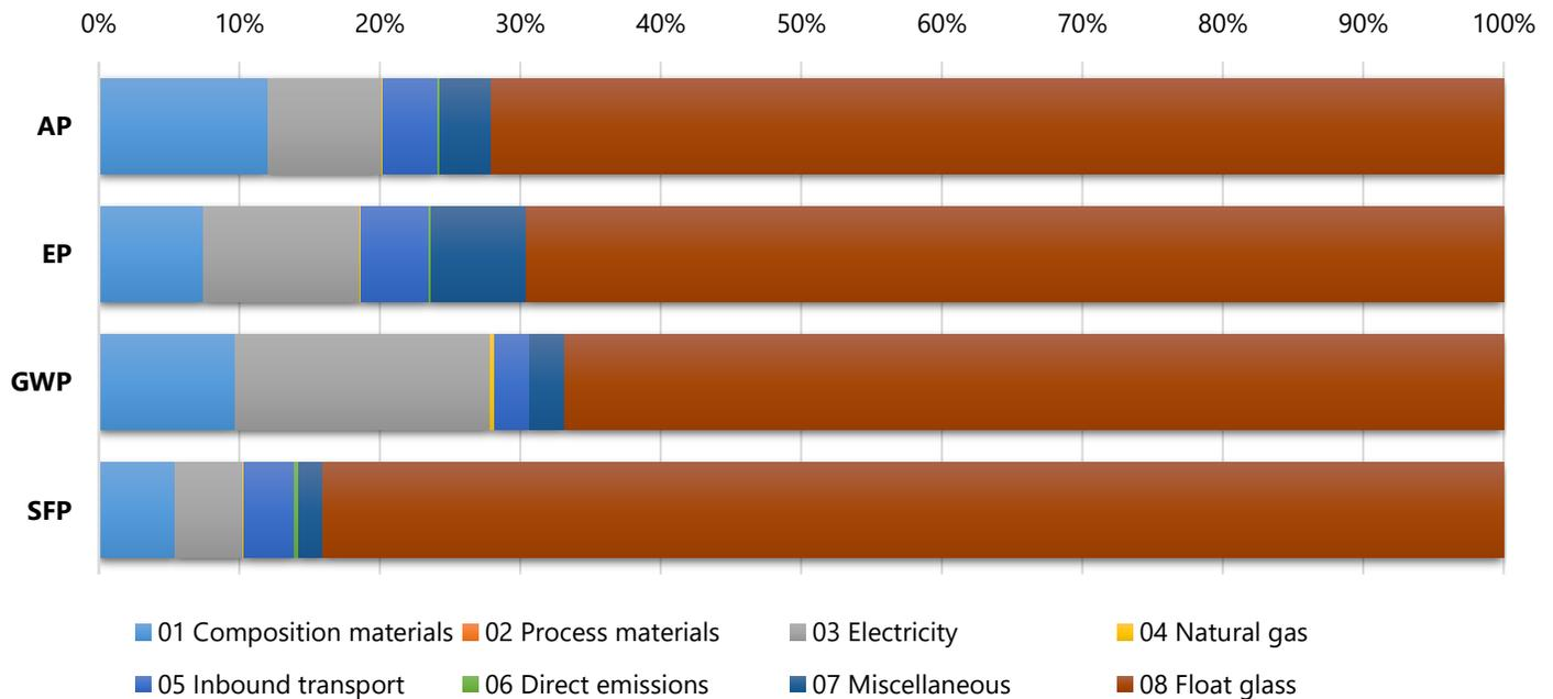
Figure 5-1: Relative contributions of uncoated glass production and the insulating process (including coating) to double pane annealed IGUs (TRACI 2.1)
