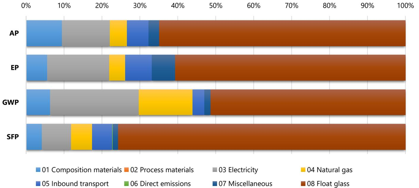
Figure 5-2: Relative contributions of uncoated glass production and the insulating process (including coating and tempering) to double pane tempered IGUs (TRACI 2.1)
