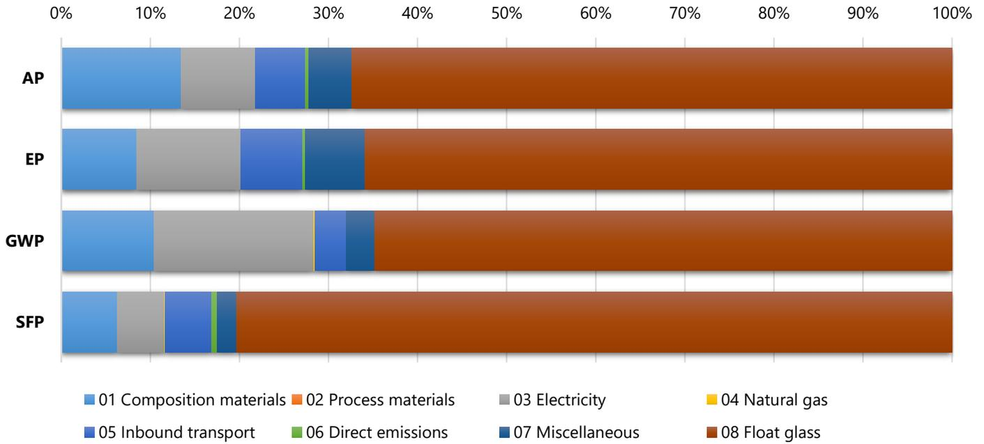
Figure 5-3: Relative contributions of uncoated glass production and the insulating process (including coating) to triple pane annealed IGUs (TRACI 2.1)
