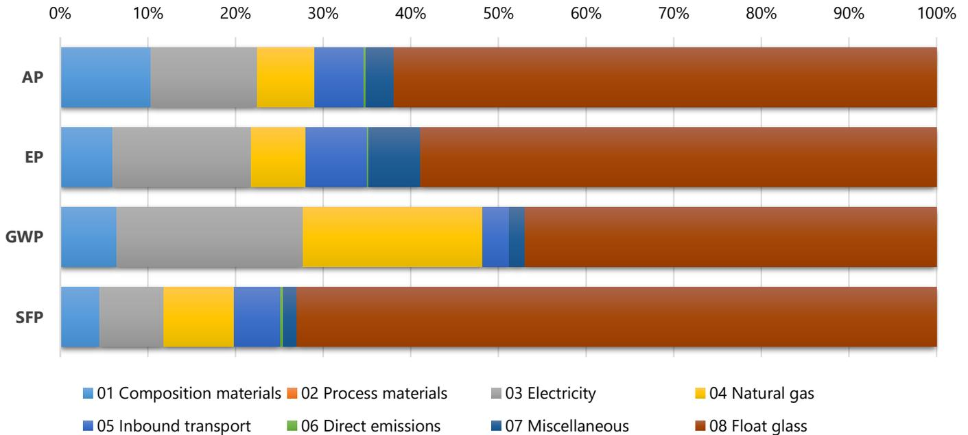
Figure 5-4: Relative contributions of uncoated glass production and the insulating process (including coating and tempering) to triple pane tempered IGUs (TRACI 2.1)
