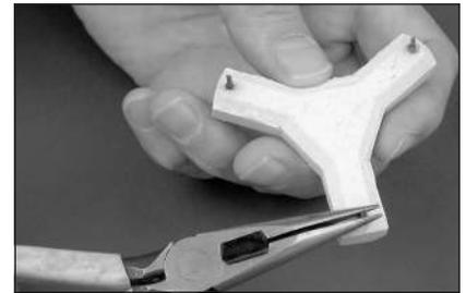
Straighten stilt pins with pliers.
