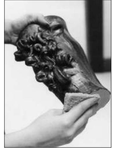
To dry foot a piece, remove all glaze from the portion of the piece that will rest on the shelf.
