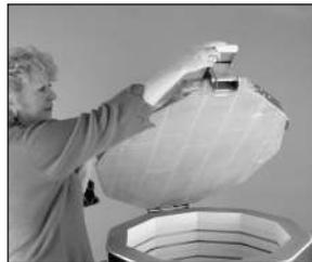
2 Do not let go of the side lid handle until the lid reaches its fully opened position. Otherwise the lid could slam upward, damaging the firebricks near the hinge. (Please note: This type of damage is not covered by warranty.)
