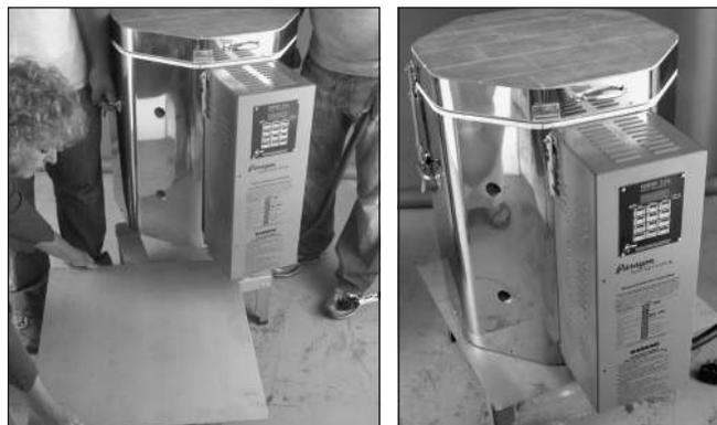
You can buy the galvanized sheet metal from a hardware store. It should be large enough to protect the entire kiln bottom.
