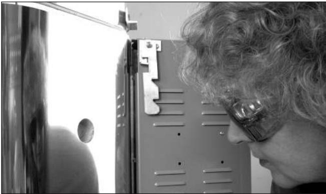
Wear firing safety glasses when viewing a witness cone.
