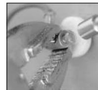
Installing the element connectors.
