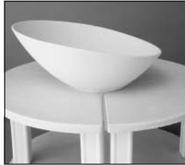
Half shelves increase kiln space by making it possible to fire tall pieces on one side of the kiln and one or more layers of small items on the other side.
