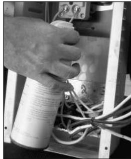
Cleaning the switch box with canned air.
