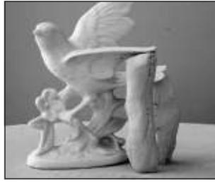
Rolls of porcelain clay are used here to support a delicate piece.
