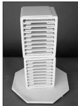
Tile holders are a special type of kiln furniture. They make efficient use of kiln space and allow air to circulate around tiles for even heating, thereby reducing tile warpage and cracking. Tile holders can be stacked inside the kiln.
