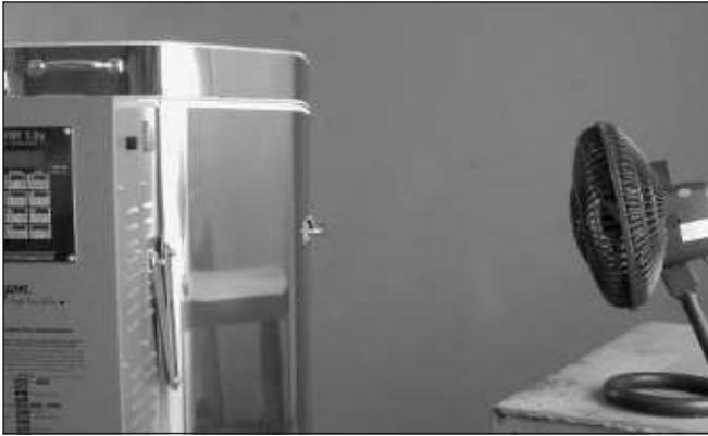
Lower the switch box temperature with air movement. This is especially useful during hot summers.
