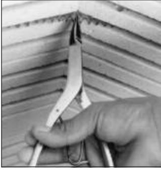
Expanding coils with automotive snap-ring pliers.
