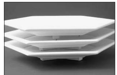
You can use stilts to separate a stack of horizontal plates. But do not stilt soft glazed pieces. Test if you are not sure.
