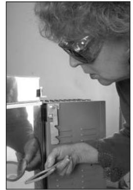
**Caution:** Some ceramists blow into the peephole to momentarily darken the cone so they can see it better. Please do not do this. This can blow brick dust onto the ware and is a safety hazard. Cool air also changes the temperature at which the cone bends.
