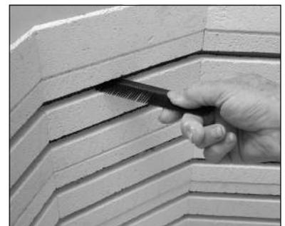
**Note:** Don't force the element into the groove corners. If the element won't fit easily, lengthen it with automotive snap-ring pliers (available from auto parts stores). Stretch the space between the
