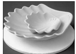
Place small, light greenware pieces directly on the floor of the kiln. Leave ample room for air to circulate around their bases since this area is difficult to heat.
