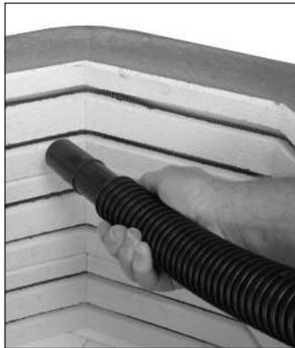
**Note:** Vacuum the kiln with a HEPA filtered vacuum cleaner or a central vacuum that takes the dust outside. Keep the vacuum hose away from the controller on digital kilns.
