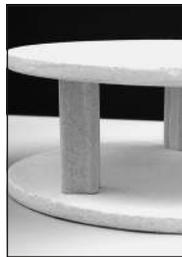
½" and 1" posts are used to obtain heights not in your post assortment. Avoid using posts taller than 10" by placing tall ware on the top shelf of your kiln.
