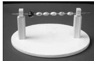
You can also center a bead rod (also called a stilt rod) over a horizontal post so that the rod extends past the post on each side. Then load an equal number of beads on each end of the rod. This is an efficient way to fire many beads since one short post can hold several rods. Be careful not to jar the kiln, or the rods could fall.
