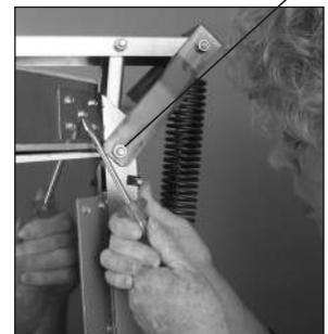
To check for play in the hinge, have someone lift the back of the lid, or lift it with the end of a screwdriver.
