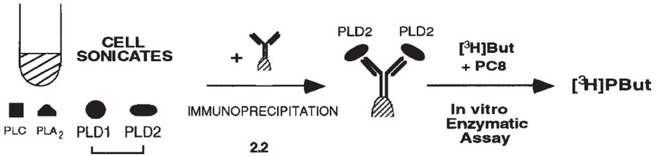
Fig. 3. Immunoprecipitation and immunocomplex enzyme assays. A specific antibody (linked to agarose beads) effectively isolates a particular phospholipase isoform (shown here PLD2) from a cell mix. The activity of the immunoprecipitated enzyme can be assayed then in vitro.
